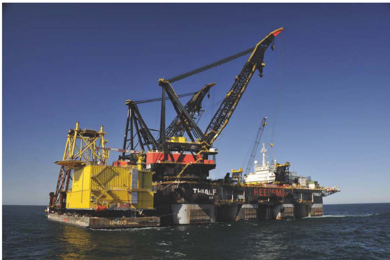
Platform installation – there are only two floating cranes in the world that can handle massive topside weights; one of them is the Thialf.
